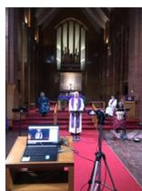
(Image 1) Laptop, one camcorder, internet cable and audio cable to the old sound board
